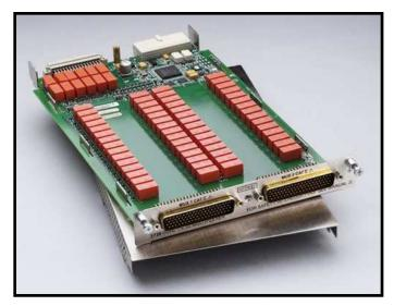
The Model 3720 offers two independent banks of  $1\times30$  two-pole multiplexers. It is ideal for general purpose switching, including temperature measurements. The two banks can automatically be connected to the Series 3700A mainframe backplane and optional DMM through the analog backplane connection relays. This connection allows the mainframe to reconfigure the card to a single  $1\times60$  two-pole multiplexer or to enable card-to-card expansion for even larger configurations.
